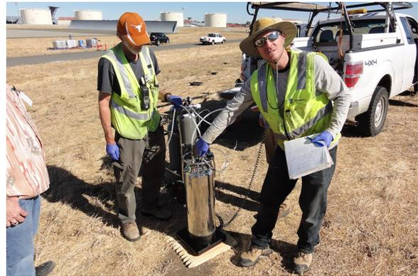
*A field technician explains the procedures for injecting a bacterial culture into a plume of solvent-contaminated groundwater without introducing oxygen into the injection point. The Travis Environmental Restoration Program will use the results of this technology demonstration at two sites (one shown in background) to guide future groundwater remediation optimizations.*
